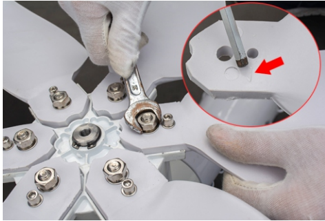
1. Let the blade cover with "Number Mark" face down, and fix it on flade plate with screws
