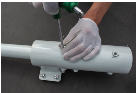
7. Fasten the three longest screws on the connecting socket
