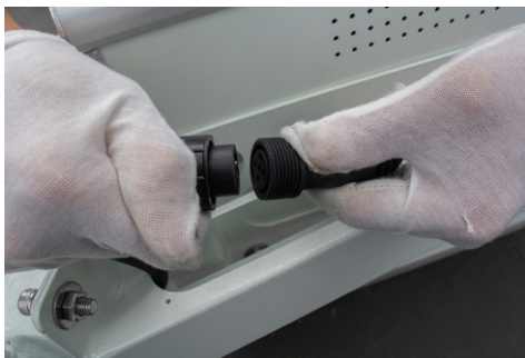
10. Open the window plate, connect the cables and connector
